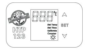
Press the Set and the Up Button together and hold for 3 Seconds to switch between the C and F temperature range. The selected will be shown by the C/F Temp Indicator.
