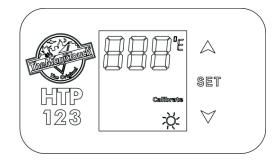
Press the Set and the Down Button together for 3 Seconds to enter the Calibration Mode. "Calibrate" will be lit. Use Up or Down Button to adjust the Value. Press Set button to quit.
