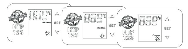
Press Set Button > 'Set Temp' will be lit > Select Temperature with the Up or Down Button > Press Set Button again > 'Set Time' will be lit > Select Time with the Up or Down Button > Press Set Button again > 'Counter' will be lit > Use the Down Button to re-set Counter to 1. Press the Set Button again to return to StandBy/Idle. If you don't need to make changes just press the Set Button again to skip the Mode. At the end all Mode Indicators must be off to return to StandBy/Idle.
