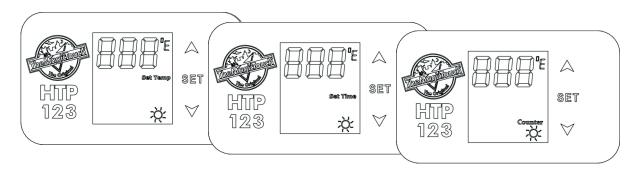
Press Set Button > 'Set Temp' will be lit > Select Temperature with the Up or Down Button > Press Set Button again > 'Set Time' will be lit > Select Time with the Up or Down Button > Press Set Button again > 'Counter' will be lit > Use the Down Button to re-set Counter to 1. Press the Set Button again to return to StandBy/Idle. If you don't need to make changes just press the Set Button again to skip the Mode. At the end all Mode Indicators must be off to return to StandBy/Idle.
