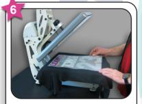
Pre press the garment to remove any creases and position the transfer.
