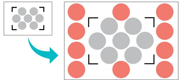
Cutting data can be placed outside the registration marks and able to make full use of the media.
