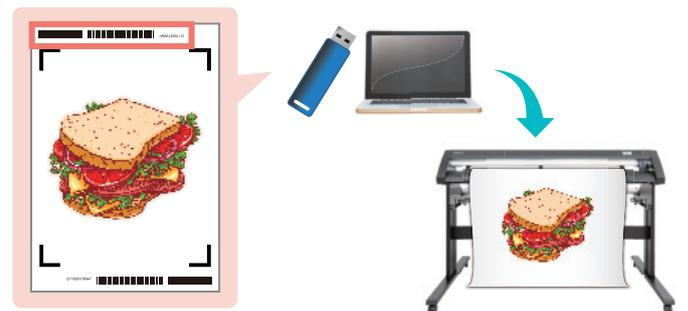
Automatic identification of cutting data with the dedicated barcode avoids cutting wrong data.
