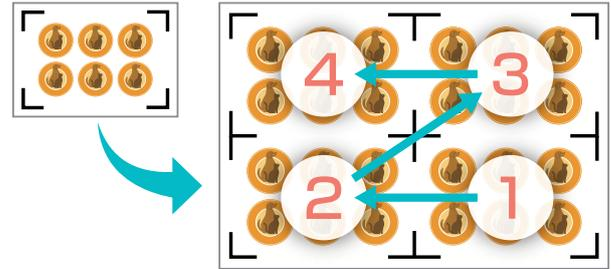
Multiple-mark compensation (Matrix copy) function supports 0mm margin.
