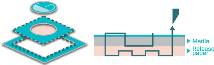
Operate both half-cut and perforation cut with one tool.
